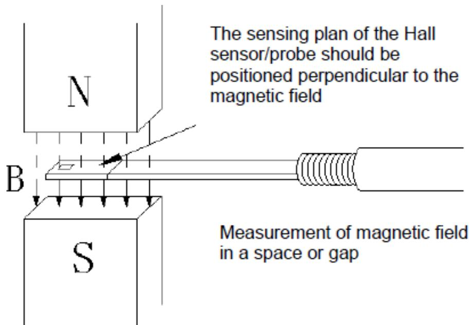
By increasing the magnetic field, a linear behavior at the voltage output should be visible.
