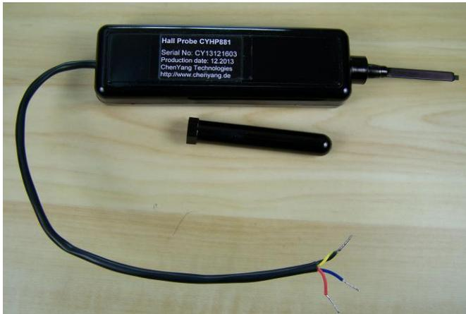
For measuring the magnetic field, please put one side of the Hall probe on the surface of the measured magnet or at the measuring point of a magnetic field carefully.
