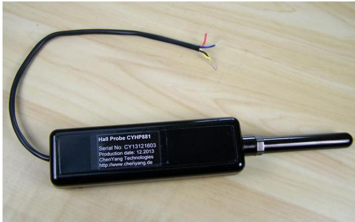
The CYHP882 is a Hall probe, which can be used to measure magnetic field strength of permanent magnet materials, electromagnets, motors, loudspeakers, magnetic sensors/transducer and other machines and instruments etc.
