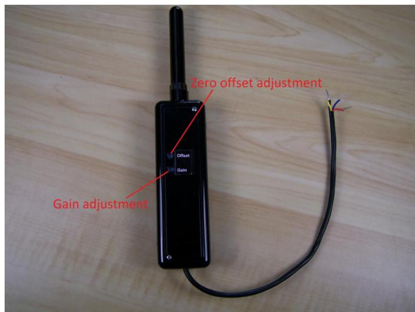
The offset can be adjusted by the potentiometer named with "Offset". It is recommended to set up the offset to about 2.5V. Then a symmetrical output range from 0.5V to 4.5V is possible.
